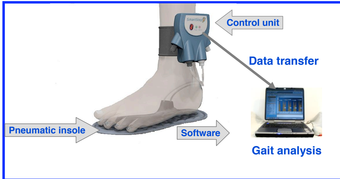
Fig 1. The computerized air-insole auditory biofeedback system (SmartStep™)
